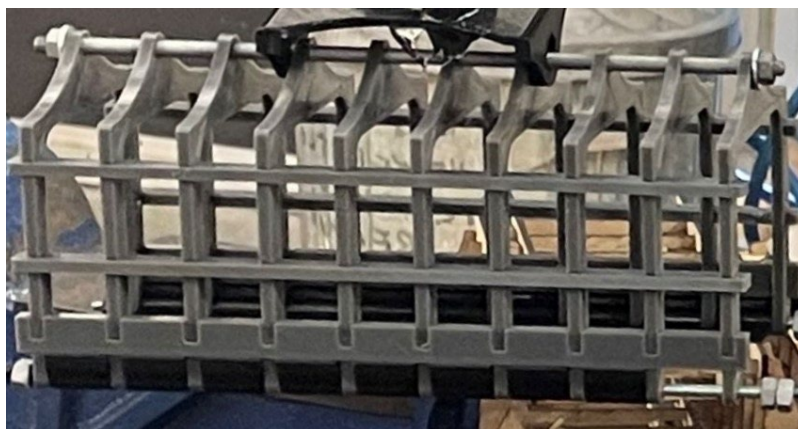
Figure 17 – Redesigned & 3D printed toolhead. Photo courtesy of Callen N.
