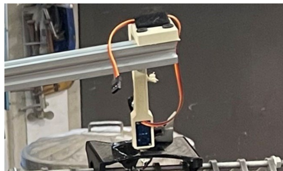
Figure 12 – Toolhead mounting bracket constructed from natural & black PLA+. Photo courtesy of Callen N.
