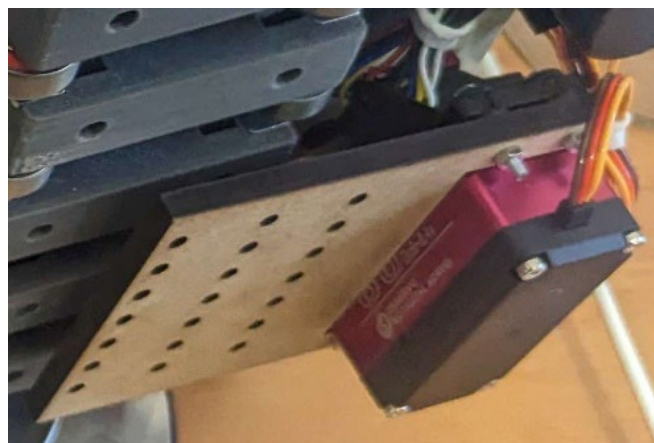
Figure 10 – MDF fixture to steel tube from vertical pivot motor. Photo courtesy of Josh Wall.
