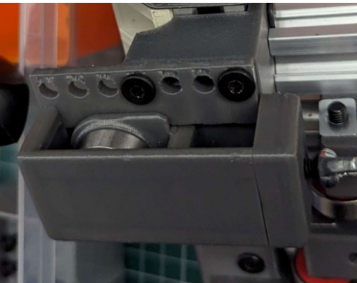
Figure 15 – (a) Linear arm at full-extension. Photos courtesy of Alec S. (b) 60 tooth belt pulley. Photos courtesy of Josh Wall. (c) Belt pretensioner. Photos courtesy of Josh Wall. (d) Belt pretensioner fitted to linear arm assembly. Photos courtesy of Josh Wall.
